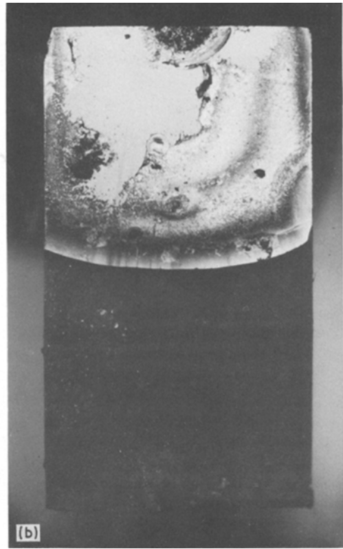
Figure 5 Typical fracture surfaces illustrating the effect of temperature on fracture surface morphology, (a) 347 K, (b) 253 K, (c) 78 K.
